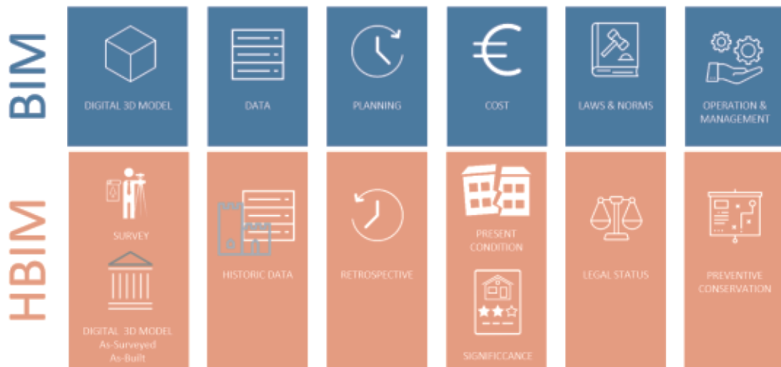
FIGURE 2 TYPE OF INFORMATION THAT SHOULD BE INTEGRATED IN HBIM DATA MODEL IN COMPARISON WITH STANDARD (SOURCE: P.JOUAN, P. HALLOT 3 )
