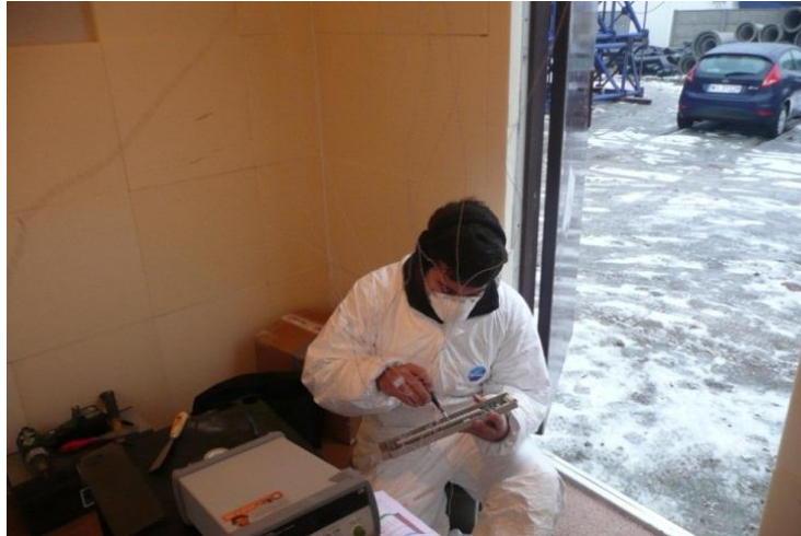
Figure 19 Thermocouples arranged in the multiplexer module at Warsaw DEMOPARK.
