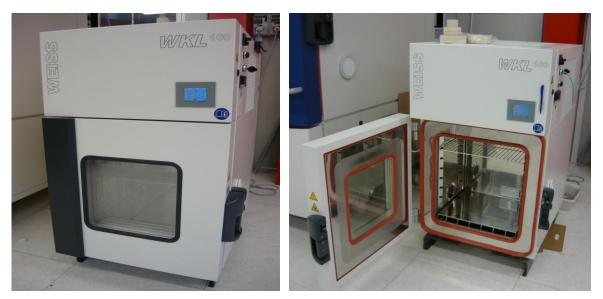
Figure 2 Equipment used for the thermal cycling tests
