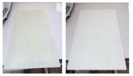
Figure 2 From the left-to-right: epoxy resin laminated using glass fiber layers ; masterbach laminated using glass fiber layers
