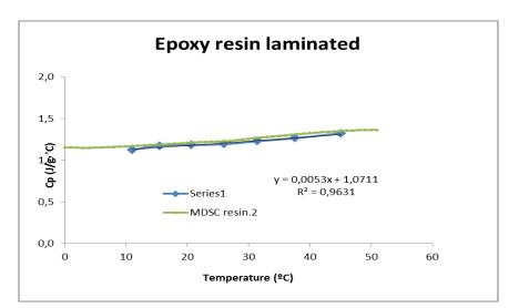
Figure 7 Heat capacity of epoxy resin laminated using glass fiber layers. The measurements were carried out using MDSC machine and a novel devide designed by UCLM
