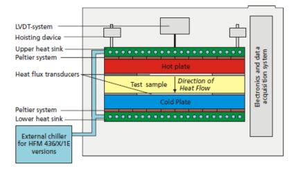
After fixing the needed parameters, the system start working, heating the upper plate and cooling the down plate.
