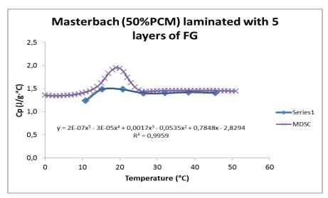
Figure 8 Heat capacity of masterbach laminated using glass fibeer, measured using MDSC and novel equipment
