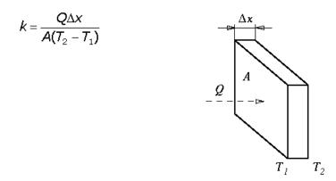
The thermal conductivity was measured using few types of equipment.
