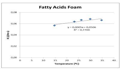
Figure 3 Thermal conductivity of PU foam containing 10% of SiO2 microcapsules confining fatty acids mixture
