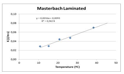
Figure 4 Thermal conductivity of laminated masterbach
