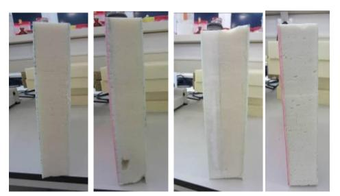
Figure 1 From the left-to-right: PU laminated; PU+masterbach laminated (laminated); PU+masterbach panel (laminated); PU+ 5% porous PCM (laminated);
