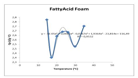
Figure 9 Heat capacity of PU foam containing 10% of SiO<sub>2</sub> microcapsules containing a fatty acids mix
