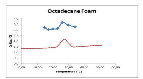
Figure 10 Heat capacity of PU foam containing SiO<sub>2</sub> microcapsules containing octadecane
