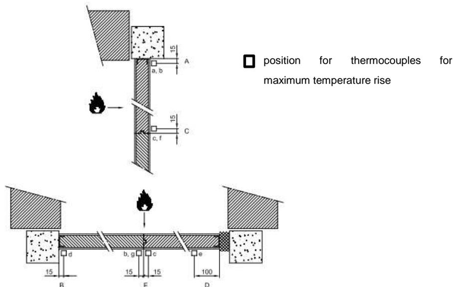
**Figure 1 Example of application points of the not exposed thermocouples in the prefabricated panels**
