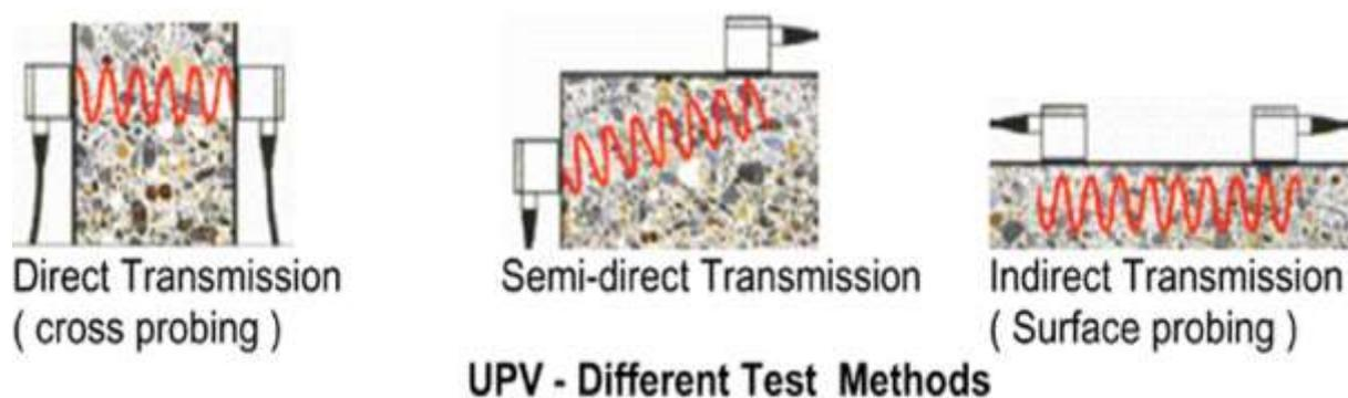
**Figure 4 Transducer positioning in UPV tests.**
