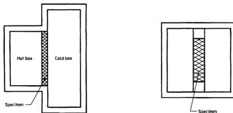
**Figure 3 Typical arrangements of the test specimen (2)**
