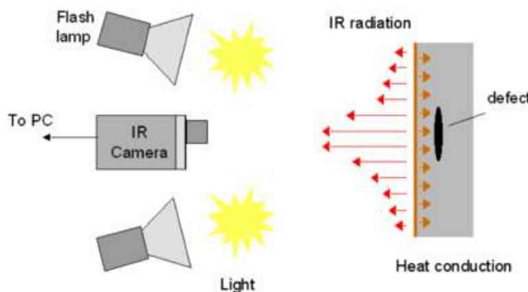
Figure 8 Apparatus for thermographic test
