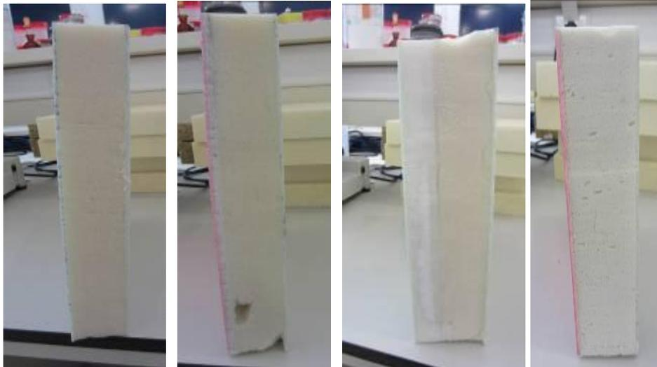
**Figure 1 From the left-to-right: PU laminated; PU+masterbach laminated (laminated); PU+masterbach panel (laminated); PU+ 5% porous PCM (laminated);**
