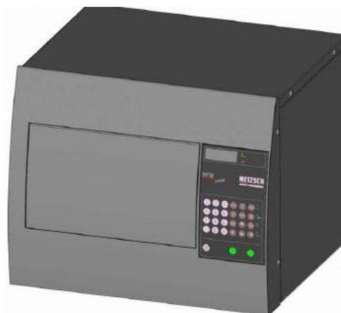
For this, samples had to be cut with dimensions 30 cm x 30 cm. Before putting in the HFM, it is necessary to know the density and include that as parameter. About the thickness, it can be introduced manually or measured automatically by the machine.
